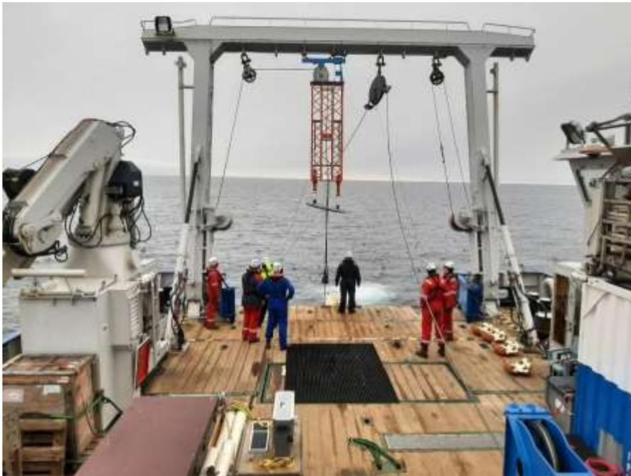
Figure 6. Deployment ROV Phoca.
