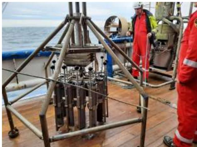
Figure 45. Multicorer on board of Pelagia.
