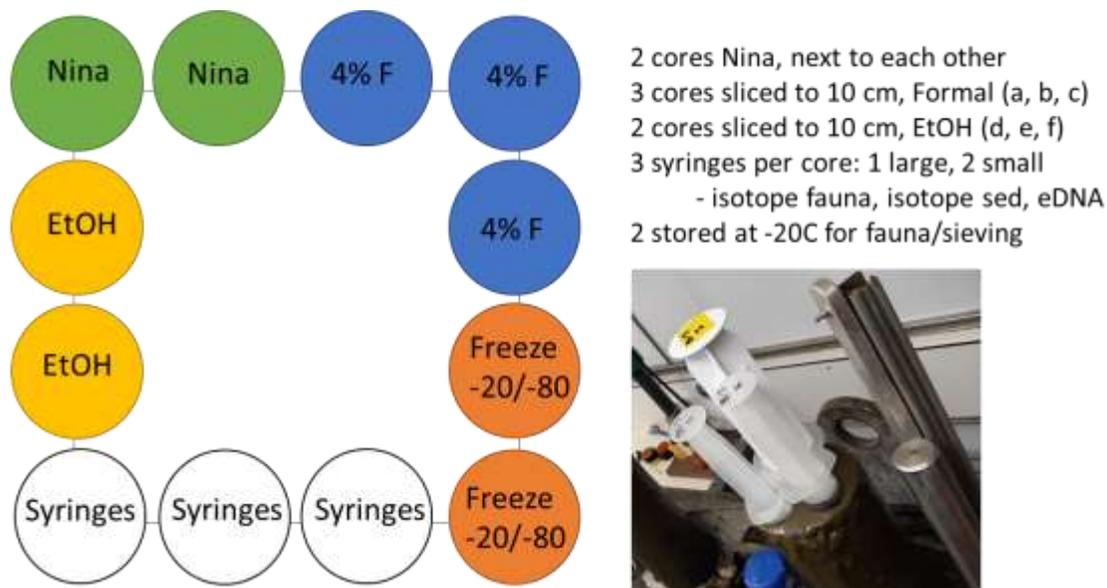
Figure 41. Sampling scheme multicorer.
