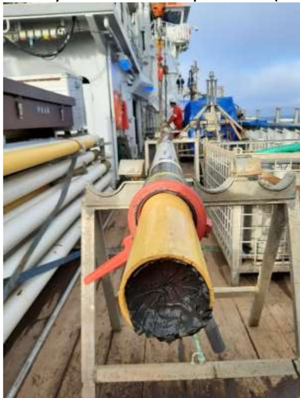
Figure 46. Piston-corer on board of Pelagia.
