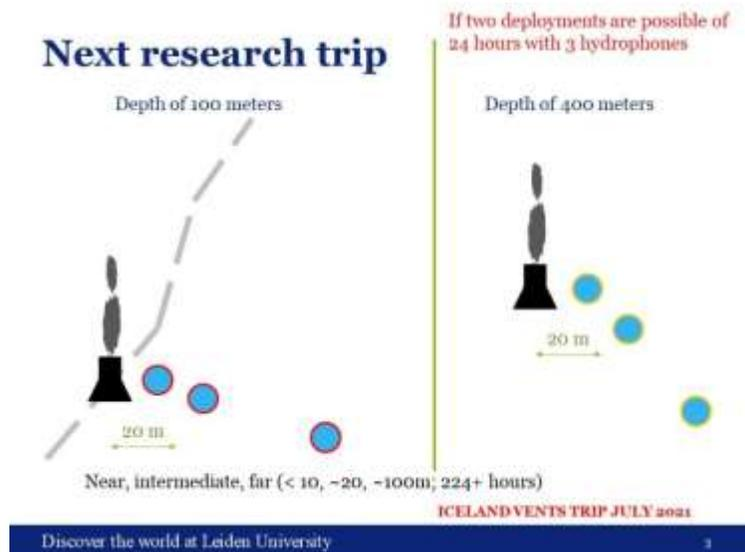
Figure 117. Schema for deployment hydrophones
