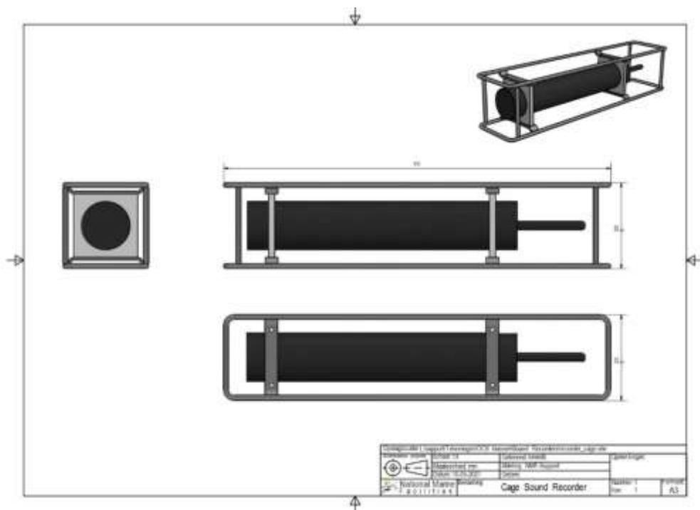
Figure 118. Cages for hydrophone deployment.
