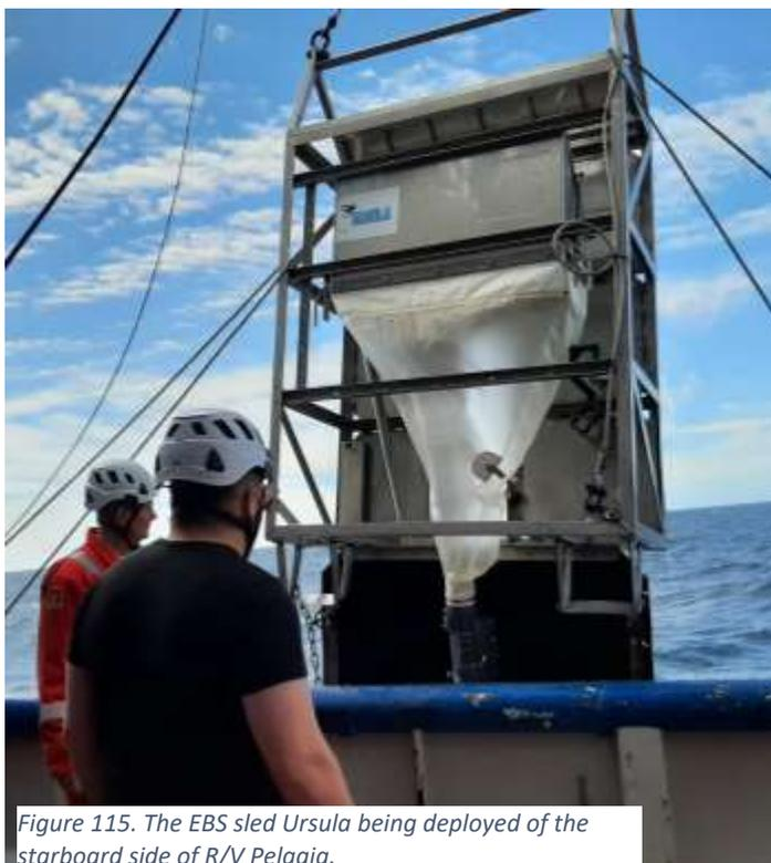
Figure 115. The EBS sled Ursula being deployed of the starboard side of R/V Pelagia.
